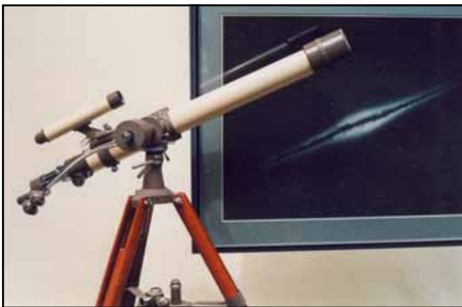
A fine pair of Swift equatorial refractor telescopes from the early 1960s. Model 831 (Serial 643117), pictured at left and assembled in position for terrestrial use, has specifications D=77\text{mm} F=1000\text{mm} ( f/13.0 ). Model 839 (Serial 60408) is smaller with D=60\text{mm} F=810\text{mm} ( f/13.5 ). Both telescopes have superlative optics. From the author's collection.
