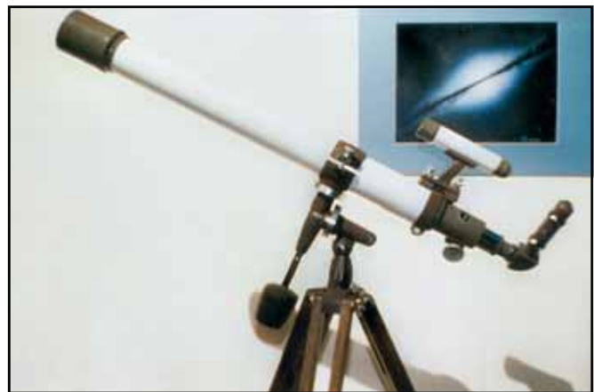
A fine pair of Swift equatorial refractor telescopes from the early 1960s. Model 831 (Serial 643117), pictured at left and assembled in position for terrestrial use, has specifications D=77\text{mm} F=1000\text{mm} ( f/13.0 ). Model 839 (Serial 60408) is smaller with D=60\text{mm} F=810\text{mm} ( f/13.5 ). Both telescopes have superlative optics. From the author's collection.
