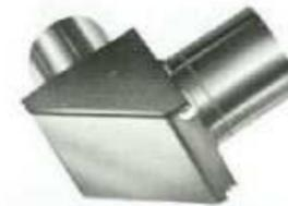
A prism eye-piece which enables you to observe celestial objects in an easy and comfortable position. The horizontal position of the object is inverted, but the vertical position is seen correctly, and, therefore, substitutes the erecting prism.
